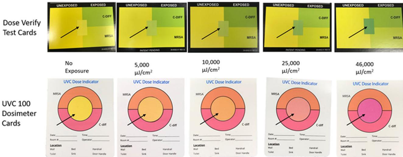
**Fig. 1.** Pictures of the 2 colorimetric indicators studied showing the color changes associated with increasing doses of ultraviolet-C (UV-C) light. Arrows point to the central rectangles (Dose Verify test cards) or circles (UVC 100 dosimeter cards) that indicate the level of UV-C exposure.
