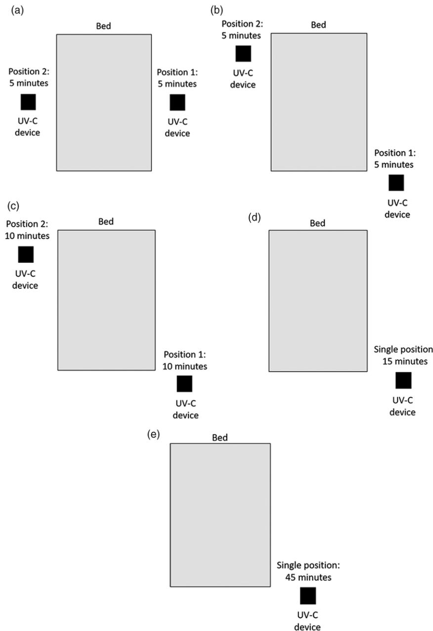
**Fig. 2.** (A–E) Illustrations showing the 5 different variations in room decontamination device positioning and ultraviolet-C (UV-C) light exposure time that were tested in rooms of patients.
